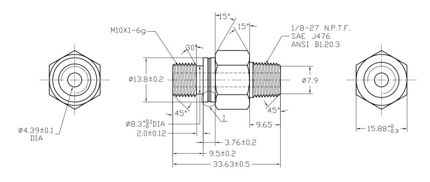
**UNLESS SPECIFIED ALL DIMENSIONS IN mm** MACHINED SURFACES Ra=3.2um ANGLE TOLERANCES ±1° **DECIMAL TOLERANCES:**
