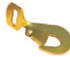
2" Twisted Snap Hook WLL: 3,666 lbs./1,666 kgs. Weight: 0.66 lbs./0.3 kgs.
