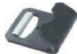
3" Flat Hook w/Alum Wear Pad, E-Coating, Black WLL: 5,400 lbs./2,455 kgs. Weight: 1.01 lbs./0.46 kgs.
