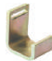
Roll-Off Hook, Yellow Zinc Plated WLL: 5,400 lbs./2,455 kgs. Weight: 1.96 lbs./0.89 kgs.
