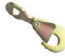
1 1/2" Twisted Snap Hook WLL: 2,200 lbs./1,000 kgs. Weight: 0.37 lbs./0.17 kgs.
