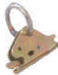
2" E & A Fitting w/O-Ring WLL: 1,666 lbs./758 kgs. Weight: 0.33 lbs./0.15 kgs.
