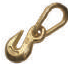
3/8" Grab Hook w/Pear Link, Yellow Dichromate Zinc Plating WLL: 5,400 lbs./2,455 kgs. Weight: 1.32 lbs./0.6 kgs.
