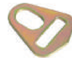
2" Flat Delta Ring WLL: 5,400 lbs./2,455 kgs. Weight: 0.28 lbs./0.13 kgs
