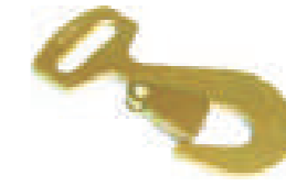
2" Flat Type Snap Hook WLL: 3,666 lbs./1,666 kgs. Weight: 0.66 lbs./0.3 kgs.
