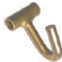
2" Tube Hook WLL: 2,200 lbs./1,000 kgs. Weight: 0.42 lbs./0.19 kgs
