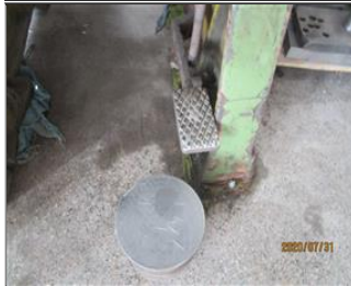
Photo of non-conformity NC-7.17 no protective cover was installed for the pedal of the punching machine.JPG
